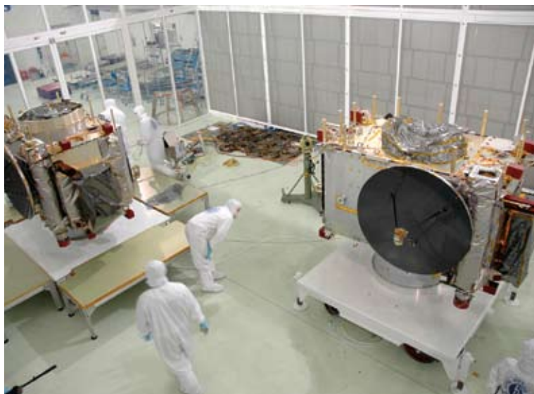
The STEREO spacecraft in Astrotech's clean room, where they are undergoing final preparations and tests for launch this summer.
